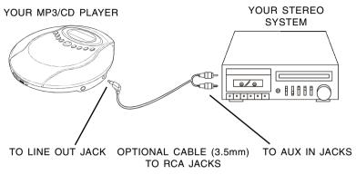
**NOTE:** Use the volume control of your stereo system to adjust the volume because the VOLUME buttons on this player have only a slight effect on the output level when used with the LINE OUT jack.
